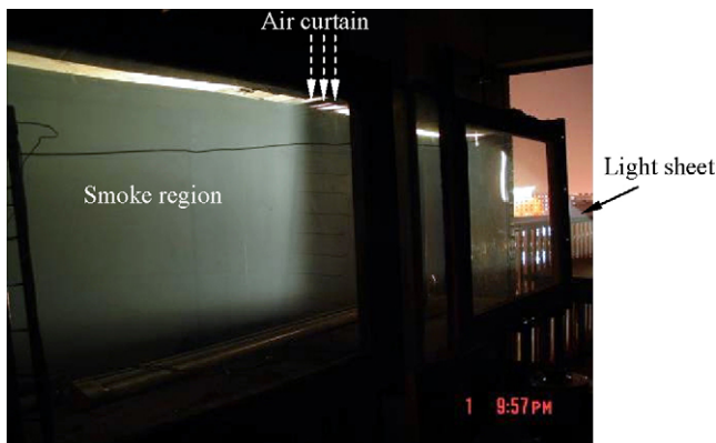
Fig. 4. Visualization of smoke confinement by the light sheet.
