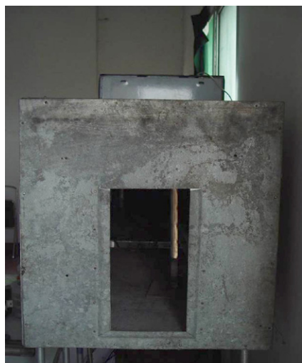
Fig. 2. Opening at the north end of the model channel: (a) photo and (b) dimensions (unit: m).
